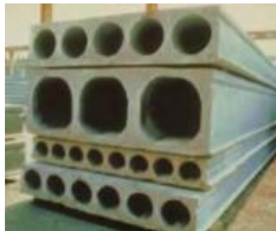
Figure 20.18 – Hollowcore Planks of Varying Thickness
